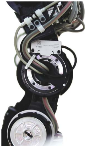
REEM-C knee joint with AksIM™ absolute rotary encoder system
