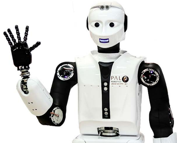
REEM-C with AksIM and Orbis rotary encoders integrated into the elbow and wrist joints.
