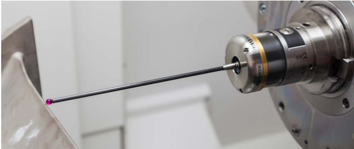
RMP600 machine tool probe locating the position of an airfoil
